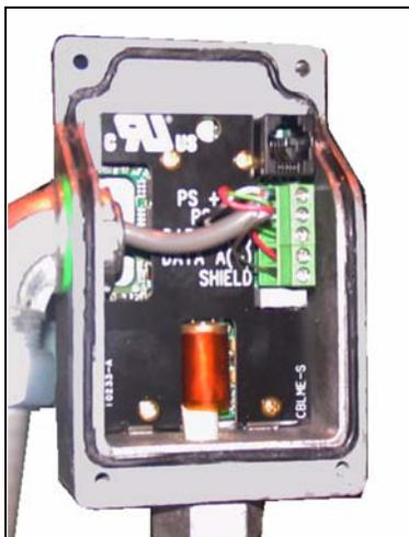
**Figure 1-2 Level Sensor Circuit Board**
