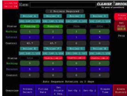
Provides Lead/Lag control for up to eight boilers when used in conjunction with the HAWK integrated boiler control system.
