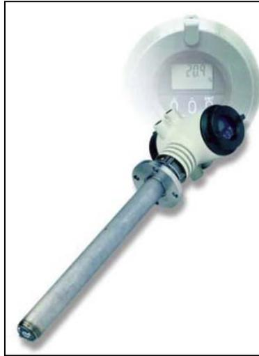
The HAWK Oxygen Monitoring System provides indication and monitoring of the boiler's exit flue gas O<sub>2</sub> concentration. In conjunction with Stack Flue Gas and Combustion Air Temperature measurements, the system also provides means for a more accurate boiler efficiency calculation.
