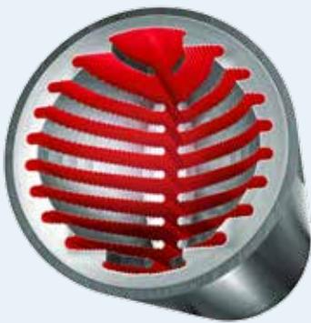
Our heat exchanger features the ALUFER firetube technology and is constructed from an inner (fireside) aluminum alloy-finned surface, die-fitted within an outer duplex stainless steel tube, providing exceptional heat exchange characteristics. The corrosion-resistant properties of the ALUFER firetube assure long life and reliability of the boiler.
